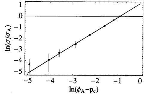
FIG. 2. Calculated values of the conductivity ratio  $\sigma/\sigma_A$  of two-dimensional, random conductor-insulator systems, where the conducting phase has conductivity  $\sigma_A$  and volume fraction  $\phi_A$ . The eight data points are taken for  $\phi_A = 1.0, 0.9, 0.8, 0.7, 0.65, 0.62, 0.61, \text{ and } 0.60$ .
