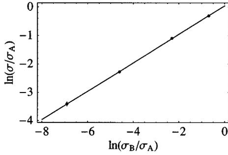
FIG. 1. Calculated values of the conductivity ratio  $\sigma/\sigma_A$  of two-dimensional, two-phase random composites, where phase A has volume fraction  $\phi_A = p_c$  and conductivity  $\sigma_A$ , and phase B has volume fraction  $\sigma_B = (1 - p_c)$  and conductivity  $\sigma_B$ . The four data points are taken for  $\sigma_B/\sigma_A = 0.5, 0.1, 0.01, \text{ and } 0.001$ .
